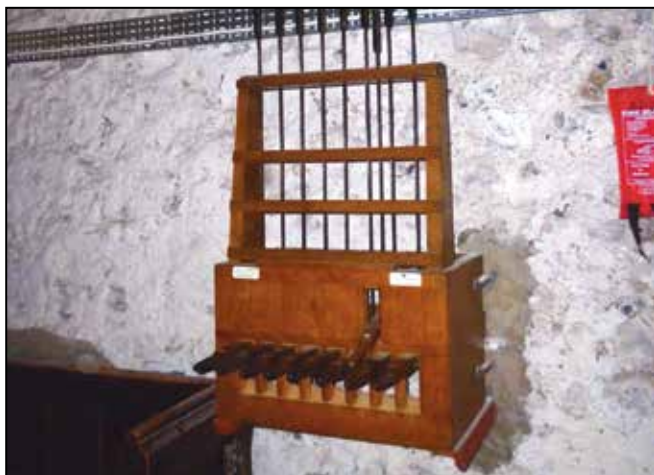
The 8 lever system for creating a tune on the bells by chiming them
