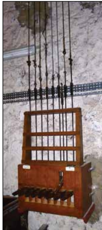
RIGHT: the lever mechanism used to chime a tune on the bells
